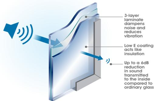
Viridian has engineered ComfortHush™ to reduce unwanted noise entering homes and buildings, whilst providing improved energy efficiency performance. ComfortHush™ 6.5mm provides a 6dB improvement compared to ordinary 3mm
